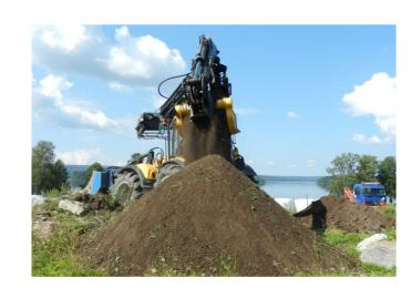
**HDX** series, largest range in the Gyru-Star compact screening family, for excavators and loaders.
