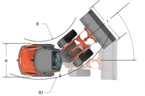
A 5250 mm B 2475 mm B1 1765 mm C 3930 mm C1 3130 mm C2 2475 mm 85 mm 670 mm 440 mm 2000 mm 1785 mm 1850 mm 1840 mm R2 3690 mm 40°
