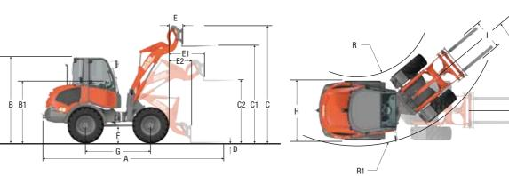
B 2475 mm B1 1765 mm C 3380 mm C1 2925 mm C2 1315 mm 70 mm 430 mm 1200 mm F2 750 mm 440 mm 2000 mm 1785 mm 1030 mm 1840 mm R1 3690 mm 409
