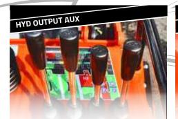
The machine provides three auxiliary outputs that allow you to use different tools at the same time.
