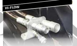
The CMF machine has a unique Hi-Flow system with two variable piston pumps with automatic constant power. This allows the machine to use the most power available and prevents the engine from stalling.
