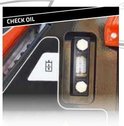
There is a single access point for checking the level, checking the temperature, and filling hydraulic oil.
