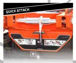
With the Cormidi Quick Attach, you can use a different attachment each time you run the machine (dumper, miniloader, concrete mixer, etc.) Simply attach, check the configuration, and use.
