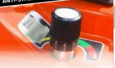
The Anti-Stall Power System guarantees excellent performance by allowing you to optimize the power of the machine while running your tools. It allows you to allocate more power to the tools with speed control, ensuring your engine never overloads.
