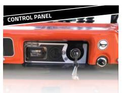
A buzzer will alert the operator in case of necessity and display always allows easy reading of the working hours.
