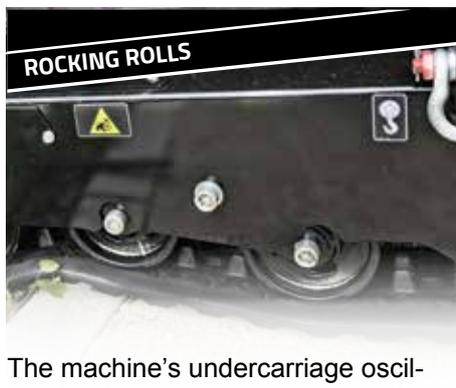
The machine's undercarriage oscillated to follow the terrain profile for increased stability and comfort.
